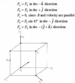
**27.6:** a) The smallest possible acceleration is zero, when the motion is parallel to the magnetic field. The greatest acceleration is when the velocity and magnetic field are at right angles:
